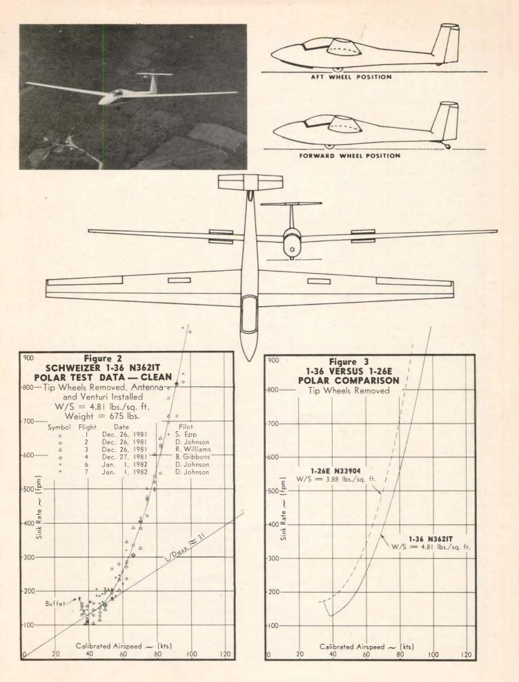
static should be used, or an additional low-error static source should be installed on the aft fuselage sides. Our test 1-36 used a factory-installed, tail-fin-mounted venturi, which worked well.
